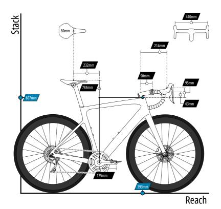
LaserX-AxisY-AxisSaddle232 mm784 mmHandlebar477 mm702 mmHoods607 mm702 mm
